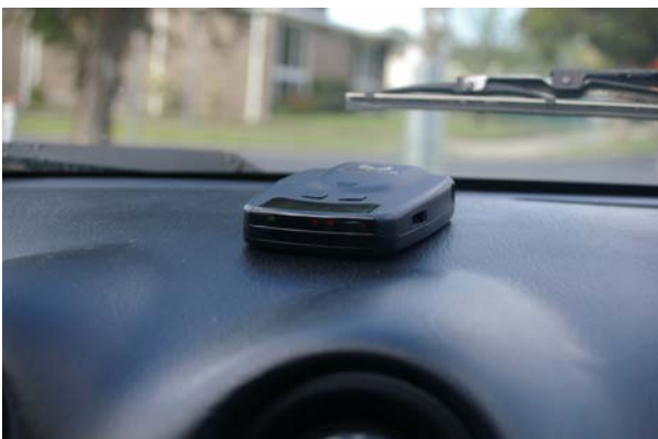
The SpeedMate in vehicle receiver collects the message from the road side transmitter and sounds a warning or provides a voice alert to the driver.
