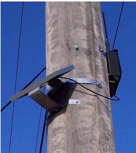
The pole mounted solar powered SpeedMate transmitter is an example of a 24 hour a day, seven day a week data transmission unit now in operation.
